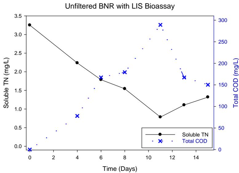
**Figure 2. Changes in total COD and soluble total nitrogen during the bioassay. One part of unfiltered CAS or BNR effluent was incubated with three parts of Long Island Sound water.**
