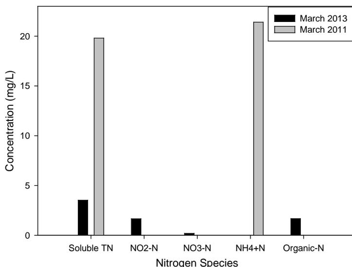
**Figure 3. Concentration of nitrogen species from all full-scale Amherst Wastewater Treatment Plant in March 2011 and March 2013. In 2011, the plant was operated in CAS while the plant is currently operated in BNR.**
